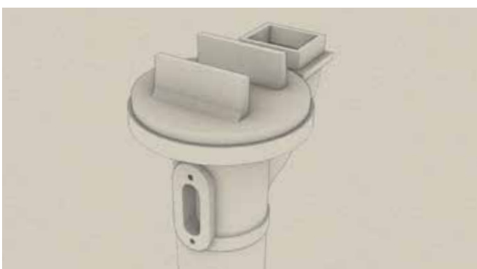
Fig.11 Model of third floor the column head at truss bearing
